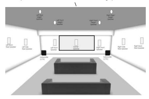
**FRONT SOUNDFIELD** – Pre wire for left, center and right front in wall speaker locations with speaker brackets. (In Wall Speaker Brackets to Be Determined)
