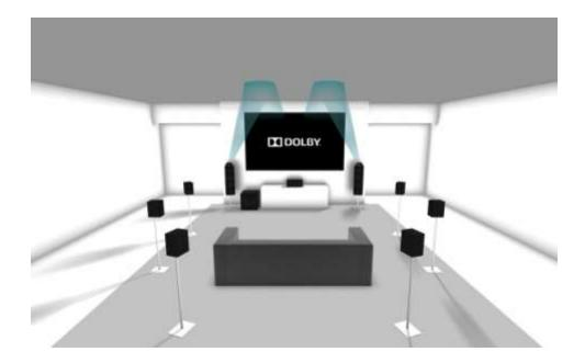
**FRONT SOUNDFIELD** – Pre wire for left and right front reflective Dolby Atmos®-enabled height speaker locations. And center speaker locations. (Floor Standing Speaker, Monitor Speaker or On Wall Speaker to Be Determined)
